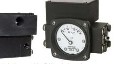
Model 140 shown with "EA" switch option. (1) Reed switch in general purpose enclosure Division 2 Hazardous locations with 7 position terminal strip. An opening at rear of enclosure accepts 1/2" flexible weather-proof or conduit connector (supplied by customer).
