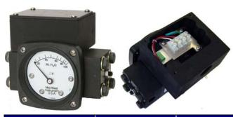
Model 140 shown with "TT" switch option. (1) 4-20 mA Transmitter (8-28 VDC Loop Power) with 7 position terminal strip. An opening at rear of enclosure accepts 1/2" flexible weather-proof or conduit connector (supplied by customer).
