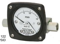
An optional maximum indication follower pointer provides automatic indication of maximum differential occurring during a time period or system cycle. Reversed pressure ports are optionally available to facilitate installation and readability depending on which side of a filter, etc., the instrument must be installed.
